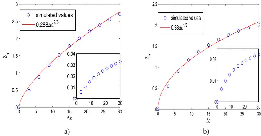
Fig. 2. Relative alignment change when applying an external bias depending on  $\Delta\epsilon$  for a)  $45^\circ$  and b)  $90^\circ$  boundary alignment. The solid curves are the fitted values. Insets show the alignment change from the unbiased case.
