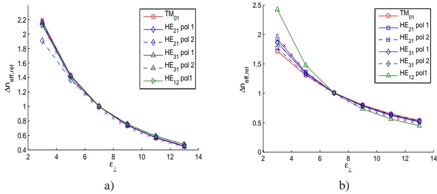
Fig. 10. Relative effective index shift depending on  $\varepsilon_{\perp}$  for a)  $45^{\circ}$  and b)  $90^{\circ}$  boundary alignment. The relative values are taken with respect to the reference configuration. The crossed lines show the fitting curves from the alignment simulations.
