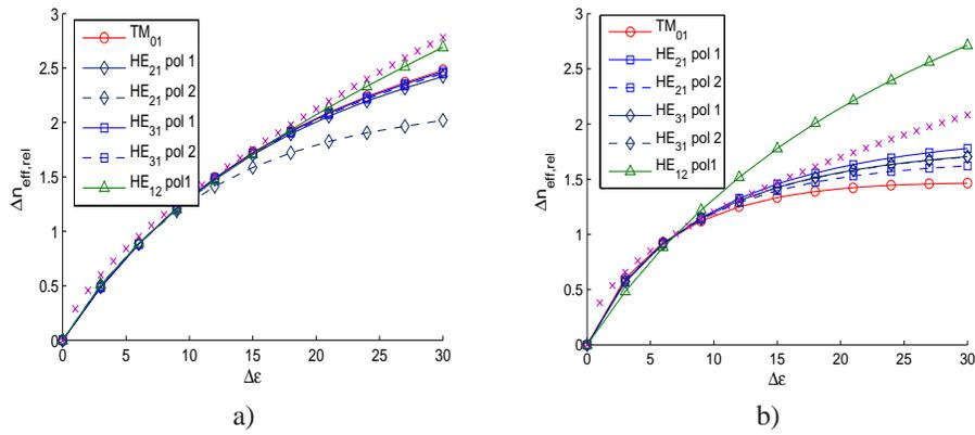
Fig. 8. Relative effective index shift depending on  $\Delta\epsilon$  for a)  $45^\circ$  boundary alignment and b)  $90^\circ$  boundary alignment. The relative values are taken with respect to the effective index shift of the modes of the reference configuration. The crossed lines show the fitting curves obtained from the alignment simulations.
