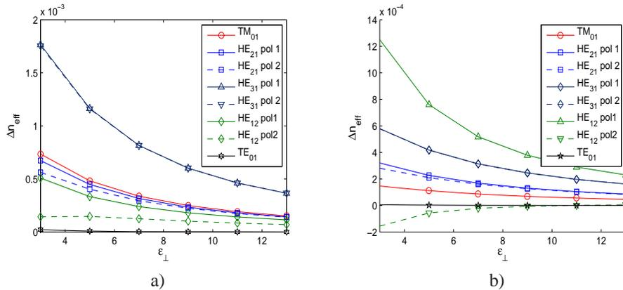
Fig. 9. Effective index shift depending on  $\epsilon_\perp$  when applying an external bias, for a)  $45^\circ$  and b)  $90^\circ$  boundary alignment. The values were taken close to the cutoff wavelengths of the modes.
