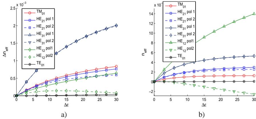
Fig. 7. Effective index shift depending on  $\Delta\epsilon$  when applying an external bias for a)  $45^\circ$  boundary alignment and b)  $90^\circ$  boundary alignment. The values were obtained close to the cutoff wavelengths of the modes.
