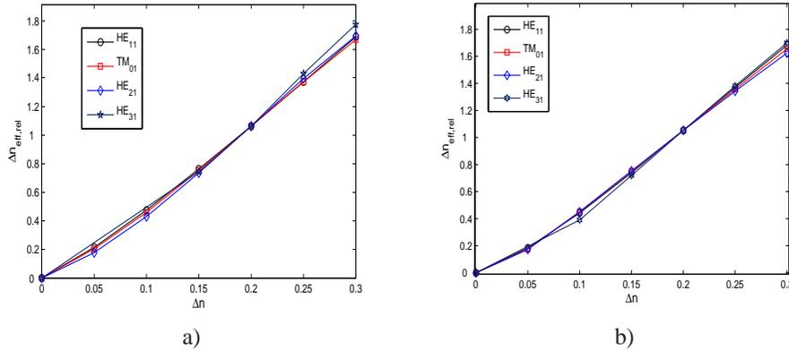
Fig. 14. Relative effective index shift depending on  $\Delta n$  when applying an external bias for a)  $45^\circ$  and b)  $90^\circ$  boundary alignment. The relative values are with respect to the effective index shift for the reference configuration.
