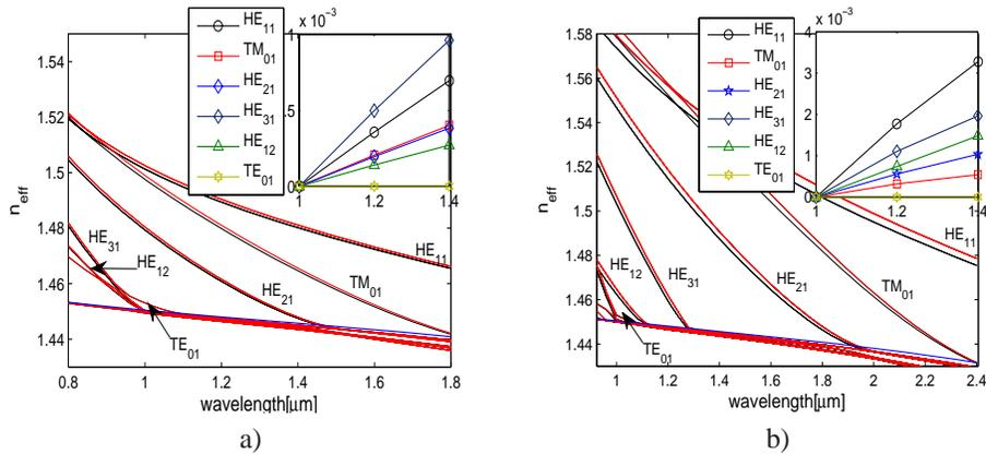
Fig. 11. Effective index plots for  $K_3/K_1 = 1$  (black, lower) and  $K_3/K_1 = 1.4$  (red, upper) for a)  $45^{\circ}$  boundary alignment and b)  $90^{\circ}$  boundary alignment. The insets show the effective index change of the y-polarizations of the modes depending on  $K_3/K_1$ .
