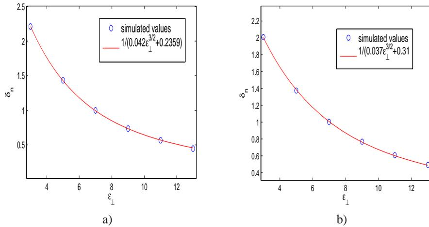
Fig. 3. Relative alignment reorientation when applying an external bias depending on  $\epsilon_\perp$  for a)  $45^\circ$  and b)  $90^\circ$  boundary alignment. The solid curves are the fitted values. The insets show the alignment deviation from the unbiased case.
