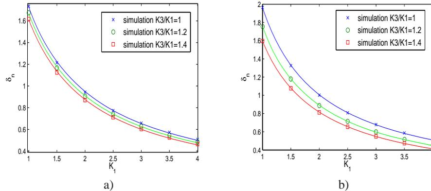
Fig. 4. Relative alignment reorientation when applying an external bias, depending on  $K_1$  for fixed  $K_3$  values. a)  $45^\circ$  boundary alignment and b)  $90^\circ$  boundary alignment. The smooth curves are the fitted values.
