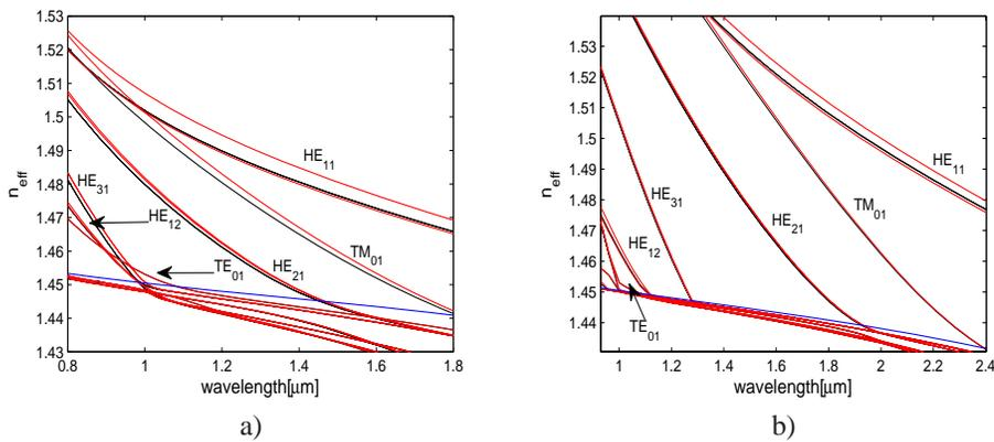
Fig. 6. Mode dispersion plots of the capillary modes for a)  $45^\circ$  and b)  $90^\circ$  boundary alignment without (black, lower) and with (red, upper) applied bias. The blue lines represent the material dispersion of the background material
