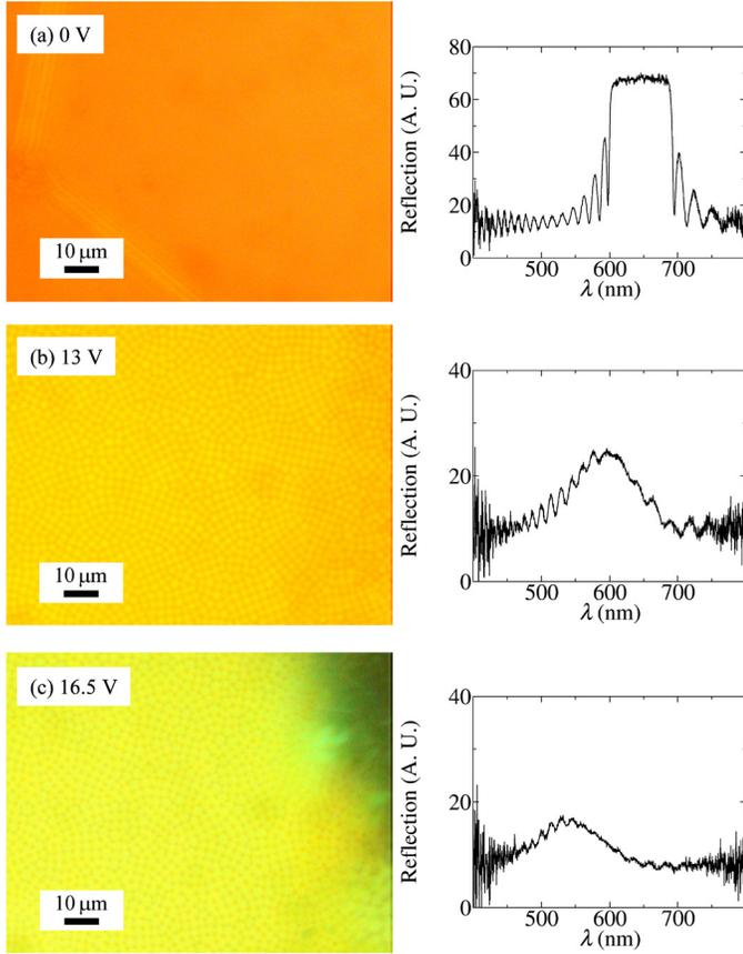
**FIGURE 1** — The reflective microscope photos (left) and reflection spectra (right) of a 5- $\mu\text{m}$  planar-aligned cell filled with a positive  $\Delta\epsilon$  ChLC at different voltages.
