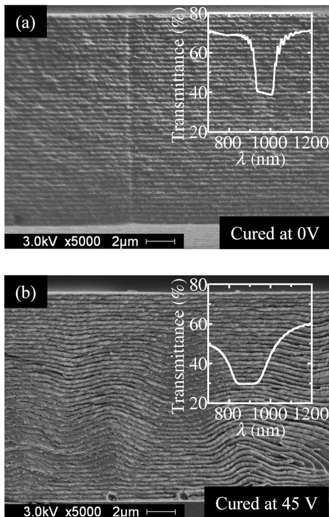
**FIGURE 3** — SEM images of a cross section of a cholesteric film cured at (a)  $V = 0$  and (b)  $V = 45 V_{rms}$ . The transmission spectrum of each film is shown in the inset.
