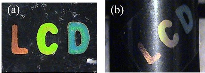
**FIGURE 4** — A three-color rollable cholesteric polymer film: (a) before bending and (b) when the film is attached to a cylindrical post holder. The “LCD” characters were exposed when different voltages were applied. The film thickness is 8  $\mu\text{m}$ .
