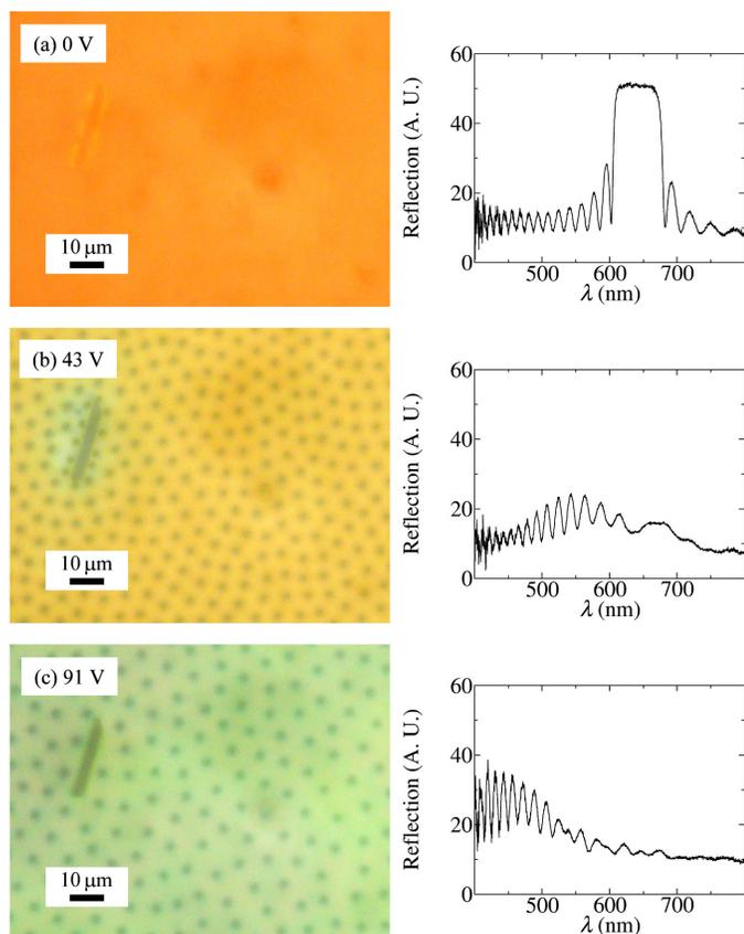
**FIGURE 2** — The reflective microscope photos (left) and reflection spectra (right) of a 5- $\mu\text{m}$  planar-aligned cell filled with a negative  $\Delta\epsilon$  ChLC at different voltages.
