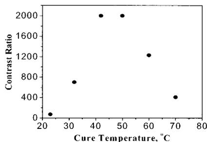
FIG. 2. The curing temperature dependent contrast ratio of the E48 LC gels containing 4% monomer concentration. Cell gap  $d = 8 \mu\text{m}$ ,  $\lambda = 633 \text{ nm}$ , and  $T = 23 \text{ }^\circ\text{C}$ .
