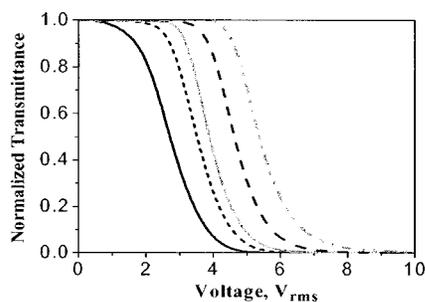
FIG. 5. The voltage-dependent transmittance of E48 LC gels with 2, 3, 4, 5, and 6 wt % (from left to right) monomer concentrations. The first-stage sample curing temperature is 50 °C. LC cell gap  $d=8\ \mu\text{m}$ , operating temperature  $T=23\ ^\circ\text{C}$ , and  $\lambda=633\ \text{nm}$ .
