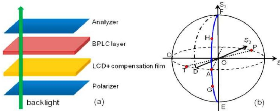
Fig. 2. (a) Device configuration for a viewing angle controllable LCD; (b) Poincaré sphere representation.
