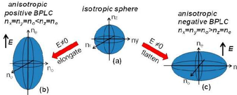
Fig. 1. Electro-optical effect on BPLC refractive index ellipsoid: (a) BPLC without an electric field, (b) positive  $\Delta\epsilon$  BPLC with an electric field, and (c) negative  $\Delta\epsilon$  BPLC with an electric field.
