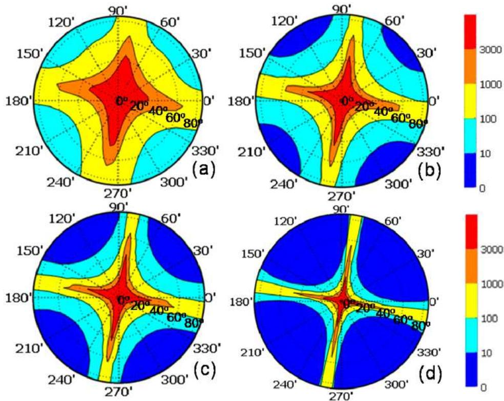
Fig. 4. Isocontrast plots of viewing angle controllable IPS cell with a negative BPLC layer at (a)  $V=5V_{rms}$ , (b)  $V=8V_{rms}$ , (c)  $V=10V_{rms}$ , and (d)  $V=20V_{rms}$ .  $\lambda=550$  nm.
