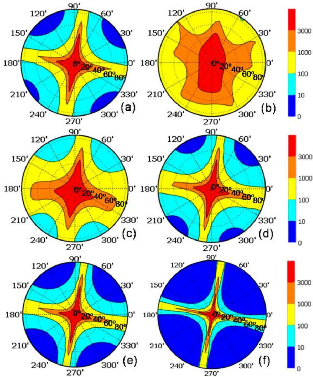
Fig. 3. Isocontrast plots of (a) an IPS-LCD without compensation film, and viewing angle controllable IPS with a biaxial film and a positive BPLC layer at (b)  $V=0$ , (c)  $V=5V_{rms}$ , (d)  $V=8V_{rms}$ , (e)  $V=10V_{rms}$ , and (f)  $V=20V_{rms}$ ,  $\lambda=550\text{nm}$ .
