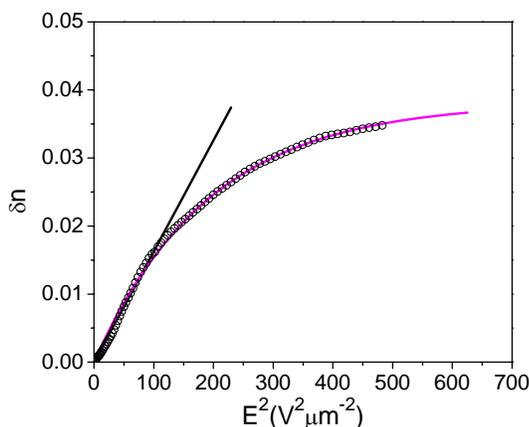
**Figure 2. Measured refractive index change (circles) and fittings with Kerr effect (black line) and extended Kerr effect (magenta).**
