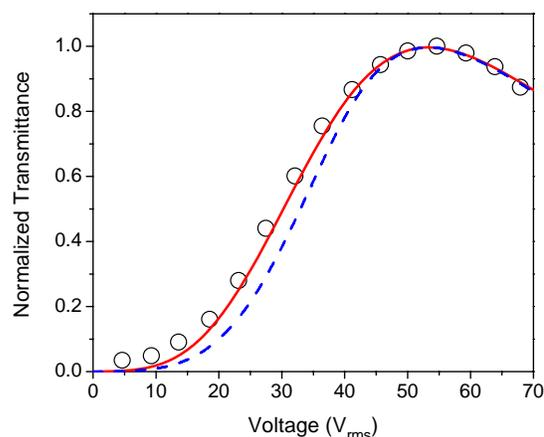
**Figure 3. Model fittings with experimental data (circles; Ref. 11) of an IPS cell using the truncation model (blue dashed lines) and extended Kerr effect (red).**
