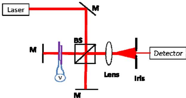
Figure 1. Experimental setup of Michelson interferometer for measuring the refractive index change of a PS-BPLC cell. M: mirror; BS: beam splitter.
